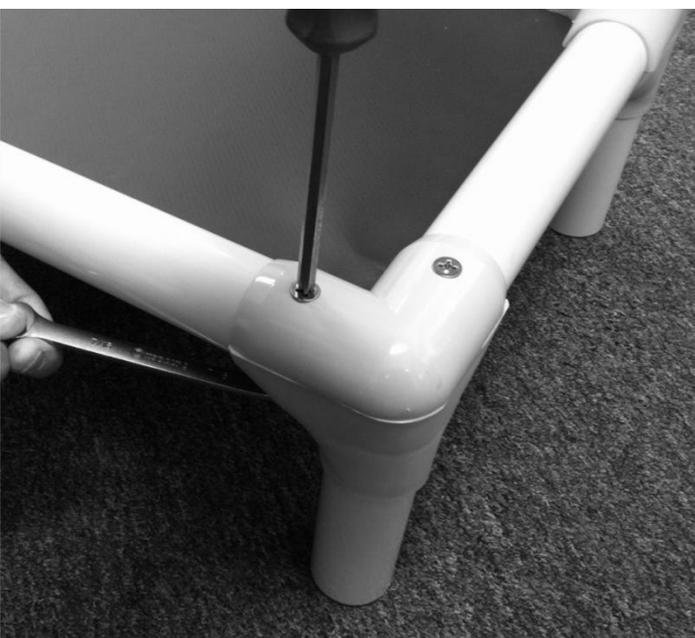
7. It is very important to properly tighten screws. Correct tightening will leave end of screw flush with the white nylon washer inside the nut.
