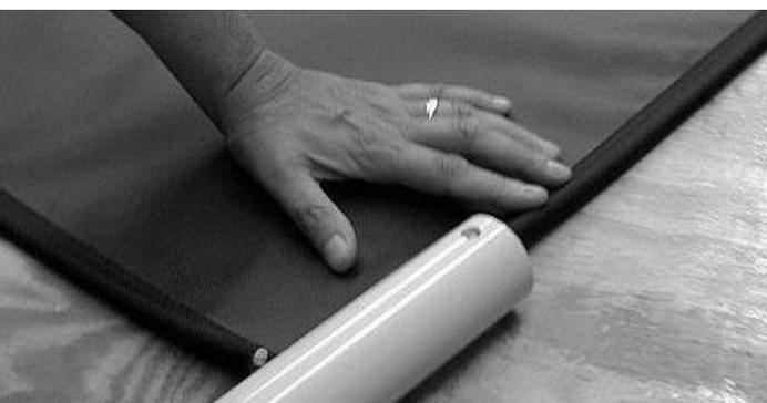
3. With the underside of the fabric facing up, position a top corner bracket beneath bed rails and insert screw through holes in each rail. (Note: Reinforcing tubes may shift inside frame during shipping and block a bolt hole. Push tube with screwdriver to recenter the pipe between holes.)
