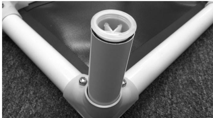
6 Turn bed over and tighten each bolt and nut on each corner.
